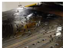
Routing and drilling aluminum sheet stacks
