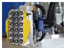
Multi-drilling “acoustic drilling” of composite nacelles
